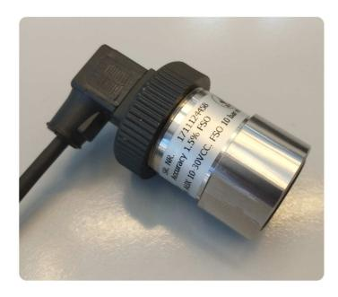
Type A transmitters are based on bridge resistance variation principle and the primary element is directly deposed on reaction mechanics by a silk screen-thick film process .
